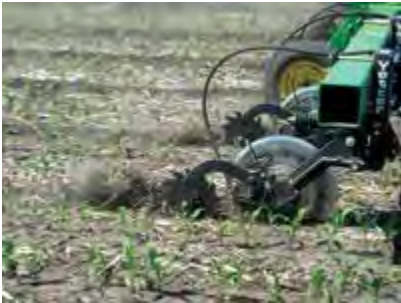
Single-disc injection coulters have low disturbance and can be operated at higher speeds.
