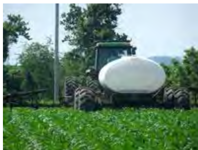
Liquid application with an All-Steer tank.
